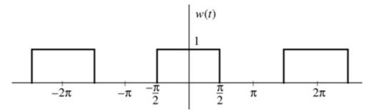
**3.** Find the trigonometric Fourier series, compact trigonometric Fourier series and exponential Fourier series for the periodic impulse train shown in the figure.
